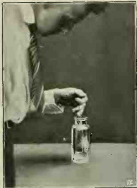
Fig. 81. Introducing Burning Sulfur In Bottle for the Minute Preparation of Sulfuric Acid—H 2 SO 4 .
