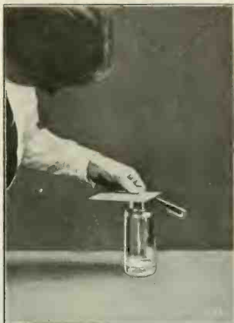
Fig. 82. Method of Introducing HNO 3 on Paper In Bottle In Which Sulfur Was Burned. For Preparation of Sulfuric Acid.
